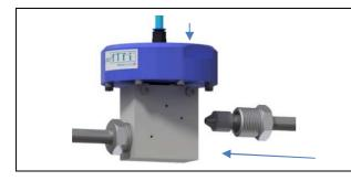
Fix pneumatic valve 2.0 with two/four screws M6 (M5 for imperial 1/4" and imperial 3/8") on the machine.
