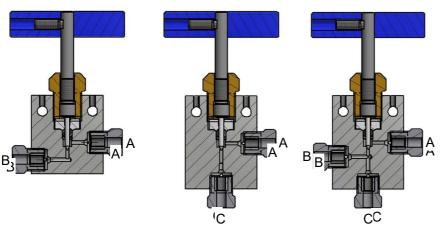
**With frequent switching** (more than one switching cycle per 5 operating hours on average), port A should be under pressure when the valve is closed. As a result, the HP seal and the valve body are subjected to static stress. The B/C connection is subjected to dynamic stress.
