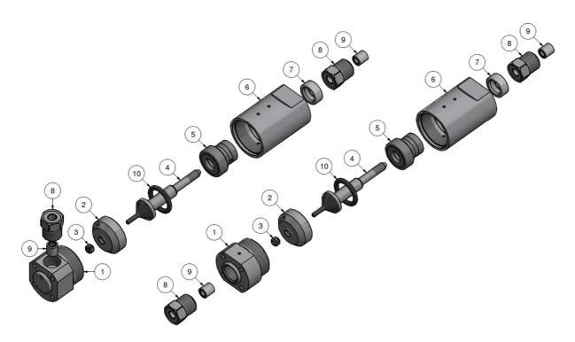
Swivel joint 921100/921100-P left and swivel joint 921000/921000-P right
